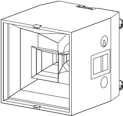
The C4-TOP is a two way horn loaded loudspeaker which provides high SPL coverage from mid to high frequencies. The constant directivity design of the C4-TOP's coaxial horns ensures that its 35° x 35° dispersion is maintained down to 700 Hz. The driver complement consists of two passively coupled devices - a 12" low/mid frequency driver and a 2" HF compression driver.
