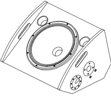
MAX is a 2-way floor monitor system and uses a 15"/2" coaxial driver combination with a passive crossover. The driver design allows the use of a compact, low height cabinet. MAX can be driven actively or passively.
